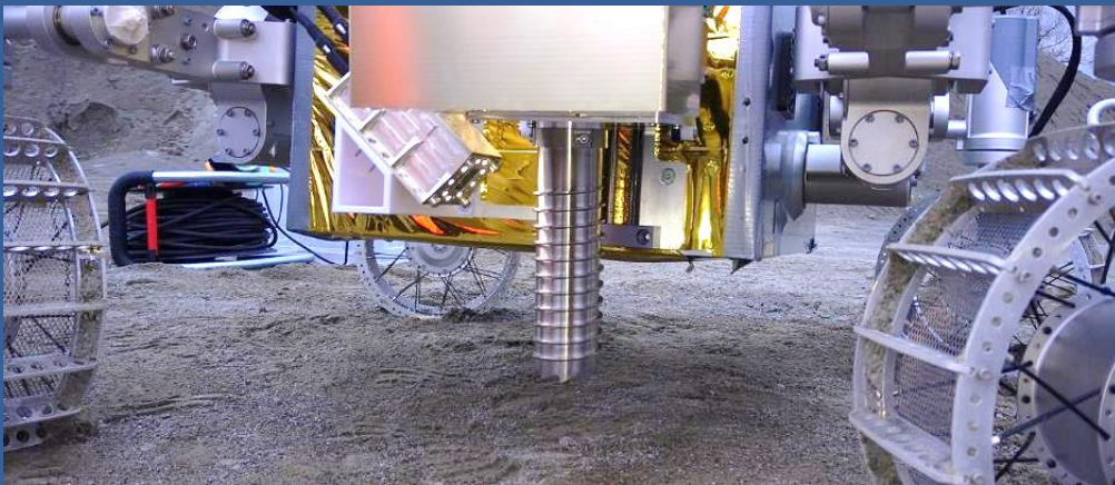
Examples of payloads mounted on front and aft bays on the LUVMI-X GM
