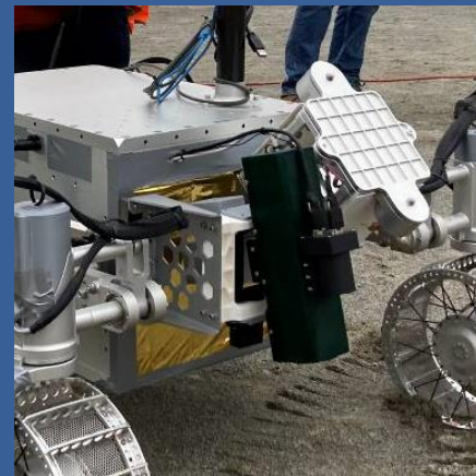
Examples of payloads mounted on front and aft bays on the LUVMI-X GM
